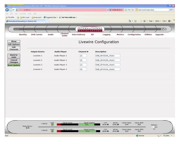
If the Pro Audio receiver is currently tuned to an active audio source, its Audio Decoder LEDs will be flashing, and the Livewire sources you have programmed are now available for automatic discovery or manual entry in your Axia network (see next step below).
