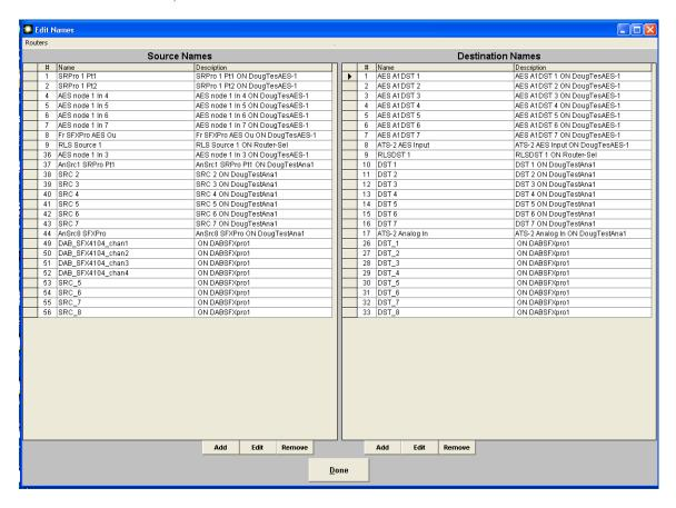
To remove entries, select each line/entry and click the associated Remove button. After removing the 12 improper entries, the example PathFinder Server names appear as indicated below:
