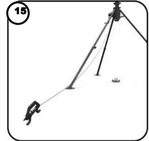
Take one **NORMAL** step for each meter of height of the mast. 10 Meters = 10 **NORMAL** Steps.
