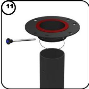
Add the red primary guy ring and pin it to the bottom hole on the mounting pole.
