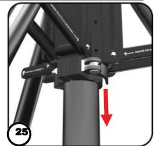
21 Raise the center mast pole until 4 inches are showing below the cam lock.
